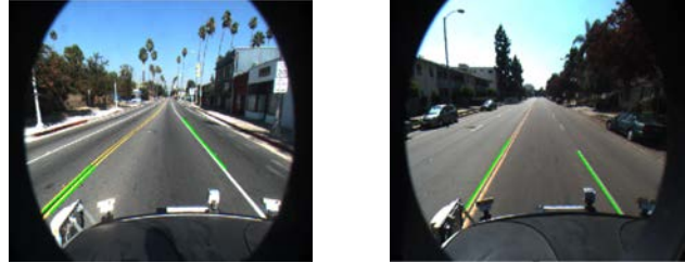
Fig.10. Examples of lane boundaries detection using segments angles computation based on Hough Transform
