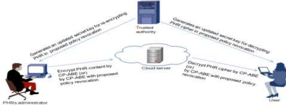
Figure 3. A scenario of PHR data sharing by using traditional CP-ABE and CP-ABE with proposed scheme
