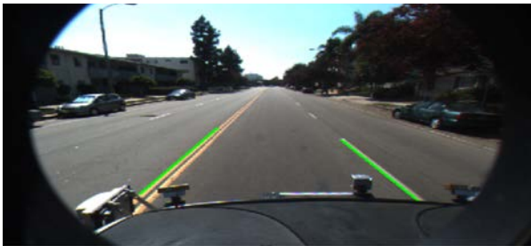
Figure 7. Detecting correct lane boundaries in original image
