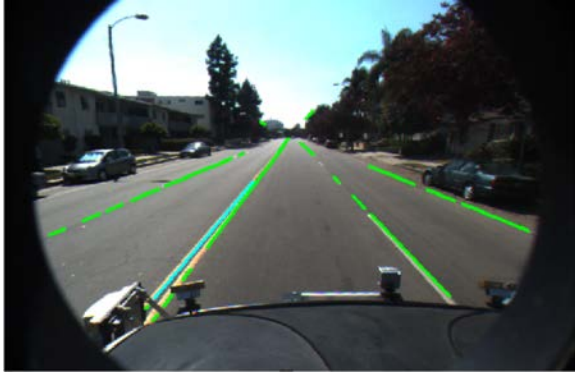
Figure 5. Detecting incorrect lines using only Hough Transform
