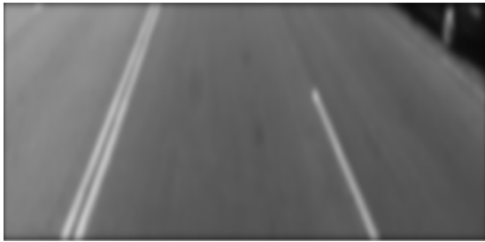
Figure 4. Denoising grayscale image using gaussian filter
