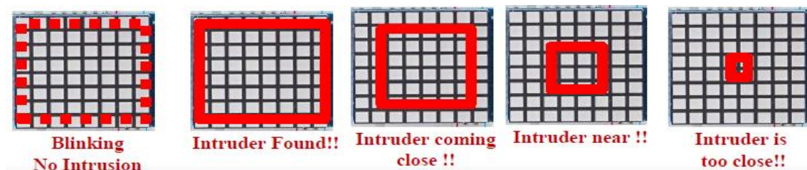
Fig. 5 Four stages on 8x8 LED display
